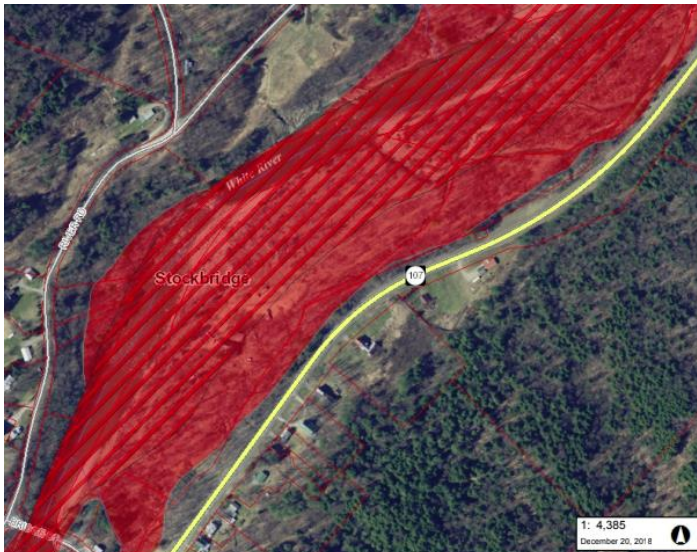
Figure 1: Floodway shown in Red Lines, Floodplain shown in red shading
